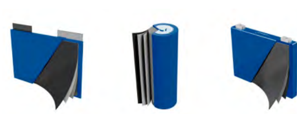
Figure 9. Typical cell types for lithium-ion batteries. From left to right: pouch cell, cylindrical cell and prismatic cell. Image source: Löbbberding et al. 2020.
