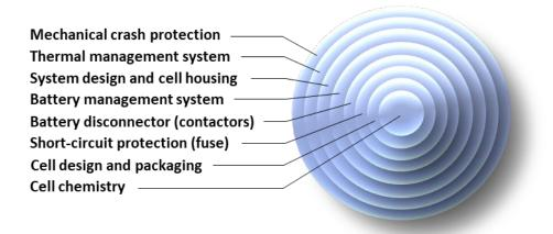
Figure 43 Schematic diagram of battery fire safety system levels for EVs. Copied from [134] [43].
