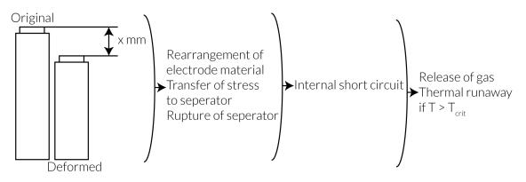
Figure 42 Mechanical deformation leading to thermal runaway [126]
