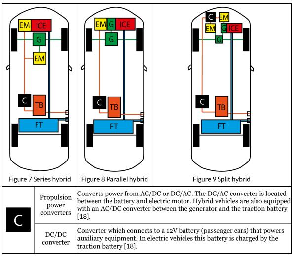
Table 5 Hybrid configurations and system components
