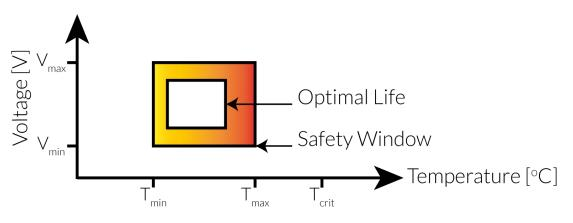
Figure 39 Illustration of the limited window of operation for a LIB cell.
