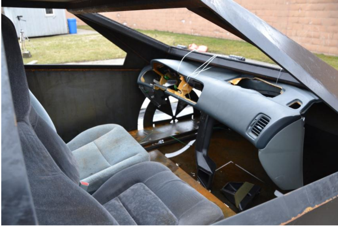
Figure 30 Dashboard and front seats installed inside the VFT for Test A3
