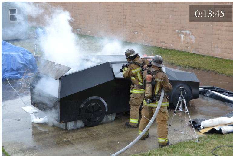
Figure 58 Test A1: Suppression starts (top left); reignition and suppression (top right, bottom left); post suppression (bottom right)
