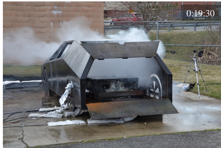
Figure 58 Test A1: Suppression starts (top left); reignition and suppression (top right, bottom left); post suppression (bottom right)
