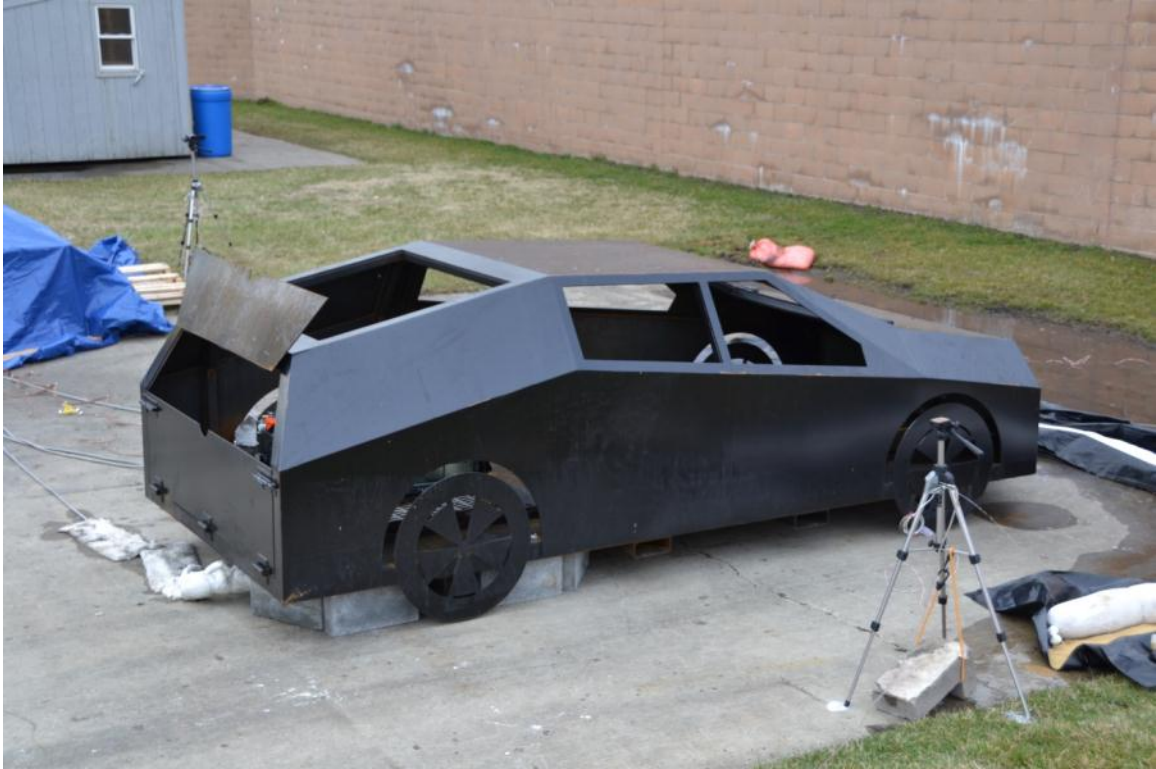
Figure 49 VFT windows were all open to air and the top portion of the back hatch was kept open to during the tests
