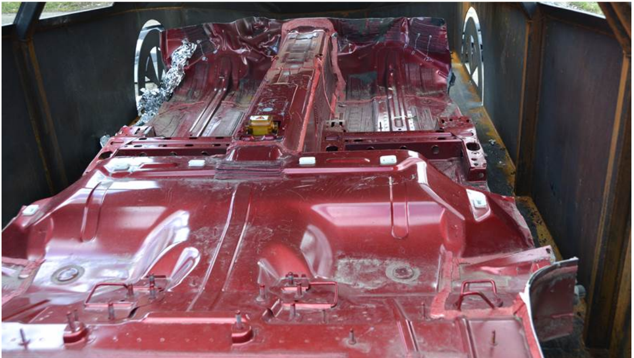
Figure 35 Top view of Battery B inside the VFT without the floor pan (top) and with the floor pan (bottom); the yellow fuse in the middle of the red floor pan is the only hole within the pan that allows for access to the battery
