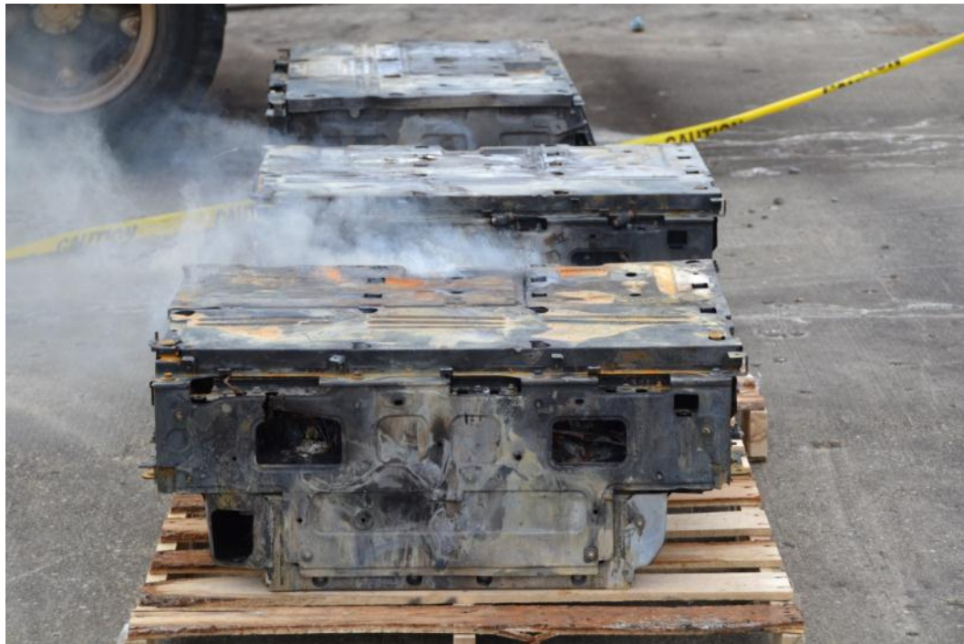
Figure 72 Off gassing of Battery A3 approximately 22 hours after the conclusion of the test
