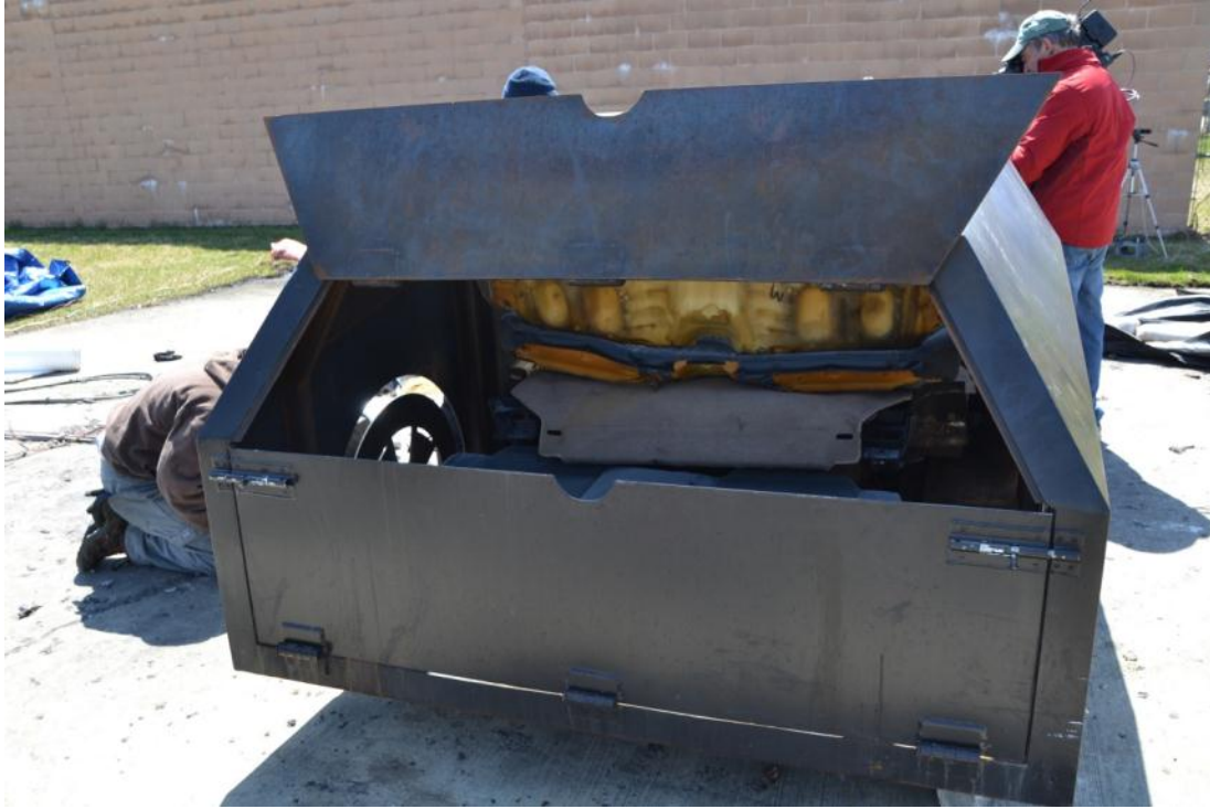
Figure 40 Back seats and carpet installed inside the VFT for Test B3
