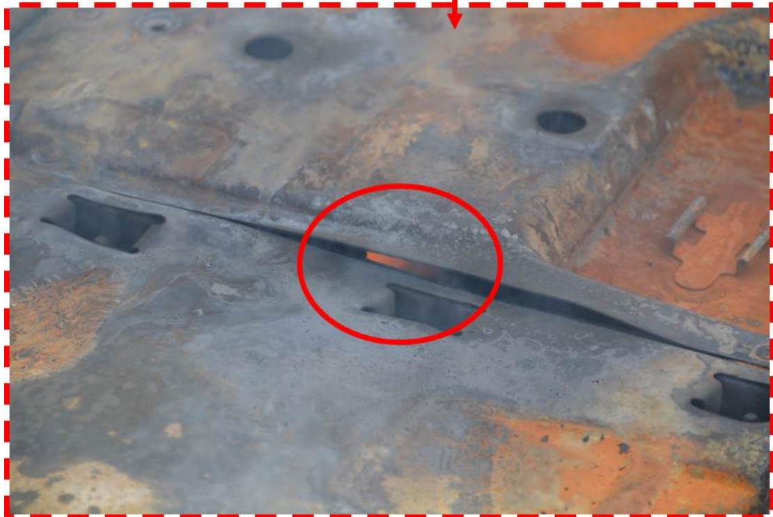
Figure 73 Reignition of Battery A3 approximately 22 hours after the conclusion of the test (flame circled red)
