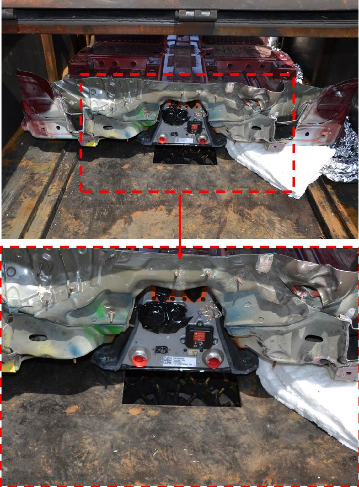
Figure 46 Connection points to Battery B once installed inside the VFT (before protection)
