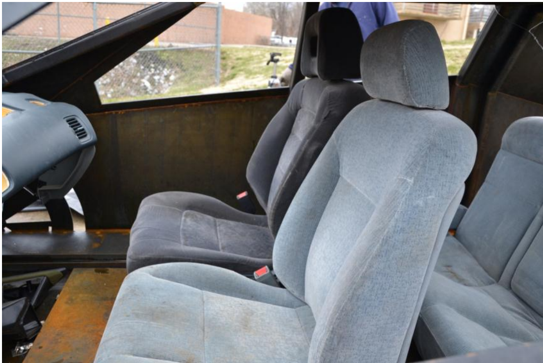
Figure 30 Dashboard and front seats installed inside the VFT for Test A3
