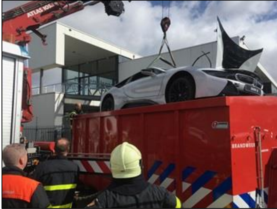
Figure 18. BMW being loaded into tank filled with water. (Source: Central and West Brabant Fire Brigade)
