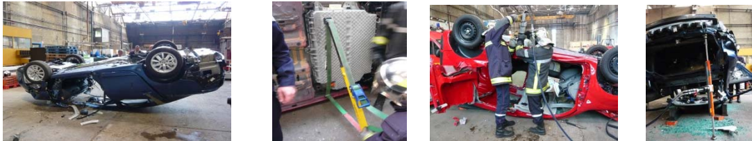
Figure 1 : a-Fluence Z.E. in balance on the roof ; b-possible wedging on Kangoo Z.E. battery ; c- no downward movement of Kangoo Z.E. on the roof ; d-possible exit of victims from Fluence Z.E. on the roof despite battery located in the trunk.
