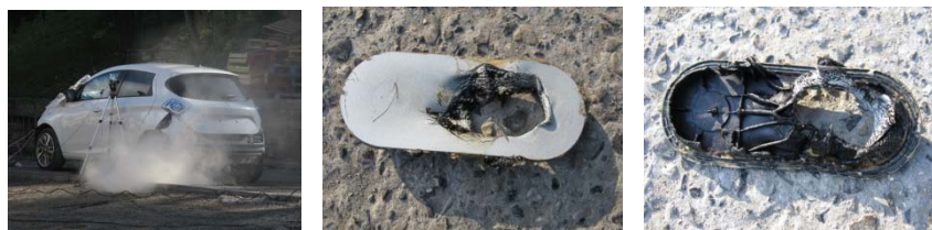
Figure 5 : a – external smokes during heat increase distribution in nearby cells of Li-Ion battery ; b & c - Fireman Access after heat increase distribution in nearby cells of Li-Ion battery.
